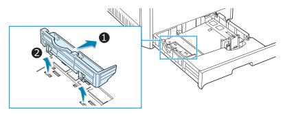
To place the paper length guide in the paper position you want, insert the locks on the bottom of the guide into the desired paper slot and push it all the way in.
